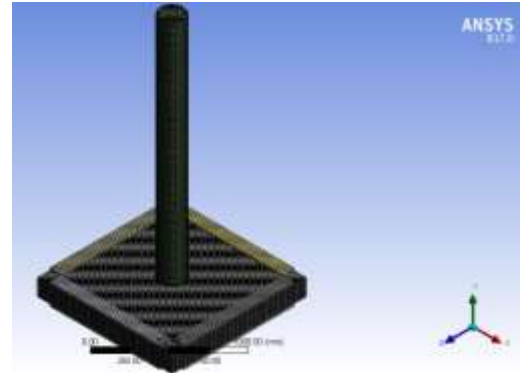
b. Meshing of the whole model including the steel impactor.
