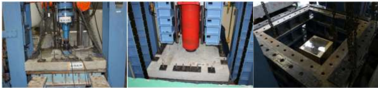
a. Rapid loading machine b. Drop weight system c. Supporting system Figure 5: Test setup of the slab specimens tested by Xiao, Li [1]
